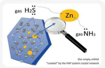
DeoHAP minerals show a porous and irregular surface able to draw with high affinity water from sweat fluids and promote a sweat drying action DeoHAP minerals neutralize malodorous gas based on ammonia and hydrogen sulfide through an optimized Lewis acid-base reaction
