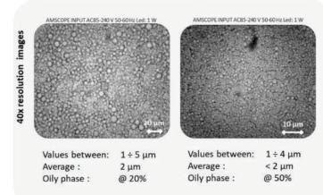
OG emulsions are micron sized systems where the oily phase is finely dispersed, to promote dermo compatibilty and silicon texture.
